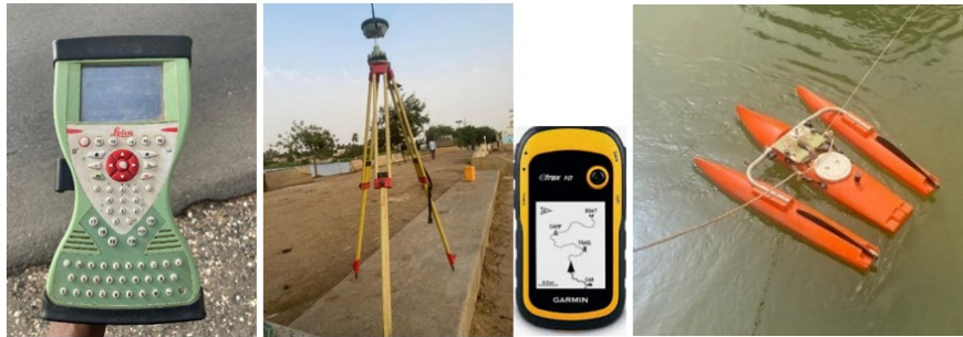
Figure 2. Equipment used (differential GPS, handheld GPS, ADCP flow meter).
